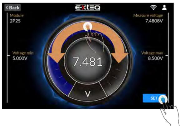
Click the center of the gauge where the value is displayed, a keypad will display to input the exact value. Confirm the value by tapping "Ok".
