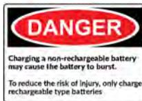
The battery contains chemicals that may generate explosive gases. Before handling the battery/module, remove all metal accessories such as rings, bracelets and necklaces.
