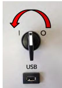
To power on, turn the switch to "I" position and hold for one (1) second.
